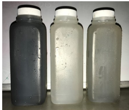
Sample bottles in Kane Drive study from left to right: conventional asphalt control, 3-inch porous overlay, and full-depth porous with underdrain.
